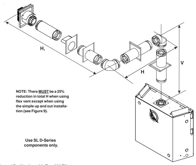
Figure 15. Venting with Two 90° Elbows
